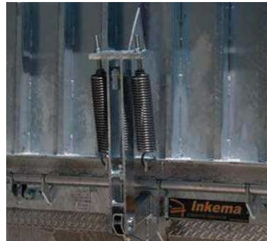
Its spring system can withstand up to 4 tons.
