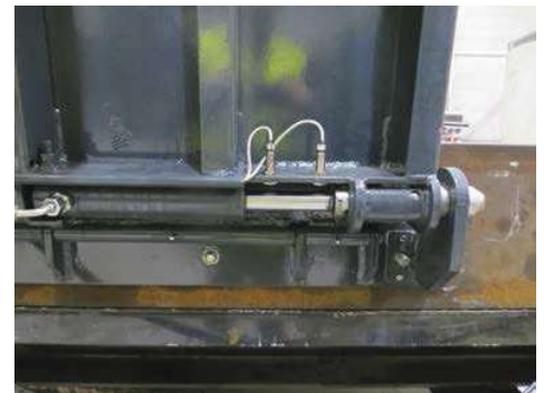
Locking system activated using safety device.
